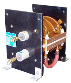
The JACKSON R.F. Transformer is an air core device designed without core material and is normally referred to as a R.F. Current Transformer. The JACKSON® R.F. Transformer is typically used in vacuum tube power supplies.
